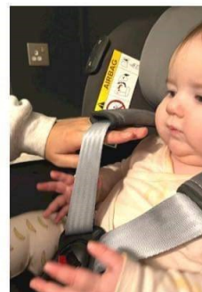
Huge gap left even though it was tight with the coat on. This is the gap that would be left when the coat compresses in a crash
